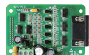
MCTC-PG-D Quadrature incremental encoder card (A, A v , B, B v ) with UVW commutation signals 5 Vdc supply, female 15-way D-type connector
