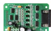
MCTC-PG-D Quadrature incremental encoder card 5 Vdc supply, female 15-way D-type connector (A, A v , B, B v , 0 V @ 5 V HTL)
